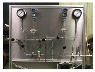
A control panel provides a precise output which is used to regulate the set point of a gas loaded relief valve.
